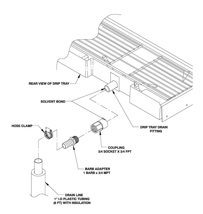
Figure 2 Drip Tray Drain Assembly
