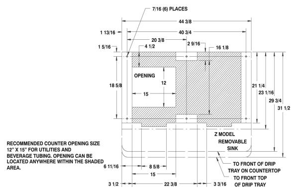
Figure 8 Mounting Template (BC models)
