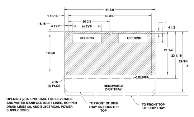
Figure 7 Mounting Template (Ice only- B models)
