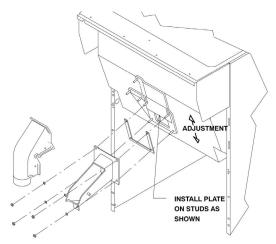
**Figure 1 Gate Restrictor Plate**
