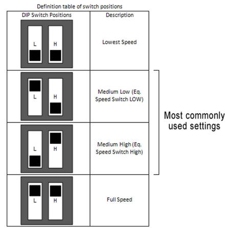
Figure 21. Motor Speed Selection DIP Switch Guide
