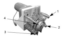
Figure 14. Pump Body Screws
