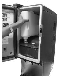
Figure 4. Loading a Concentrate Container
