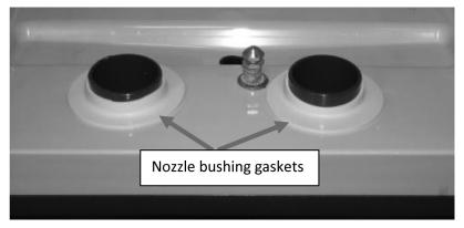
Figure 25. Nozzle bushing gaskets - proper installation
