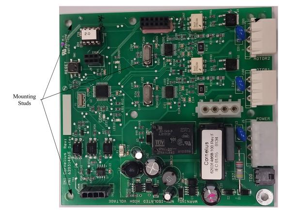
Figure 83. View of Motor Board in E-Box
