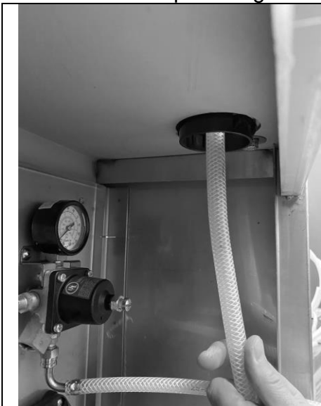
a) Route all plumbing connections to the Viper through the hole in the cart.
