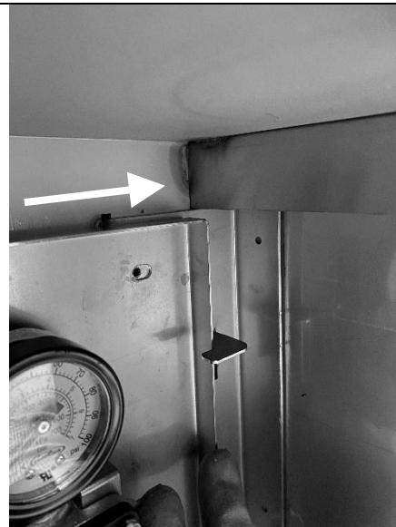
e) Slide the pump assembly to the right to engage with the upper hook.
