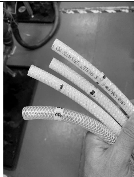
b) CO 2 and Syrup lines are labeled – the lines that run from the cart will connect to the fittings on the Viper.
