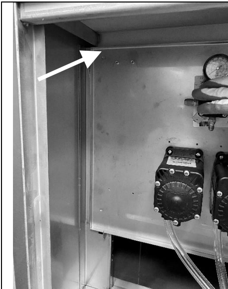
d) Rotate the pump assembly against the cart frame.
