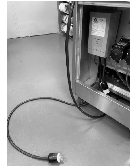
d) Route cords through the large rectangular opening at the bottom of the cart.
