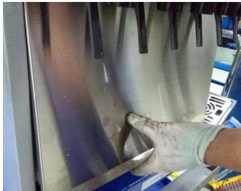
Figure 4 Remove the Splash panel
